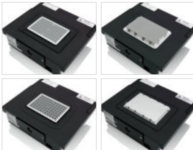
**Flexible formats.** Easily interchangeable block formats include a new Fast PCR option, standard 384-well and 96-well detection, and the TaqMan® Low Density Array block.
