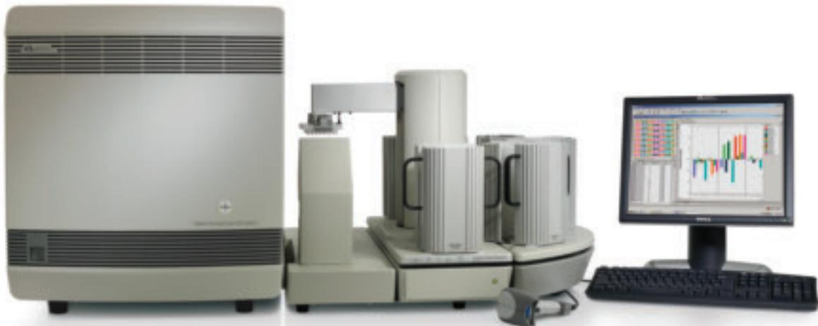
The Applied Biosystems 7900HT Fast Real-Time PCR System, shown here with Automation Accessory, is engineered from the ground up to support high-throughput applications such as gene expression quantitation and SNP genotyping.
